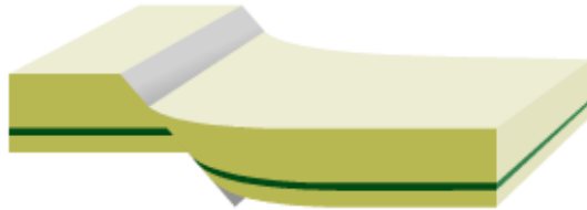
Normal fault with normal drag in hanging wall.
